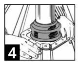
Press base to roof profile by hand.
