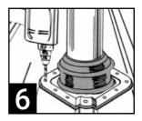
Fasten using self drilling washered screws or sealed rivets.
